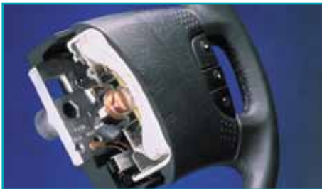
cross section front airbag undeployed
