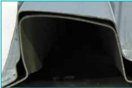
cross section B post model 1996
