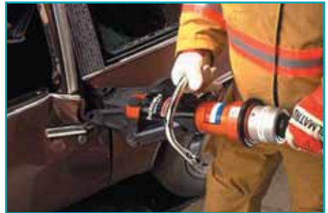
spreading a door from the vehicle
