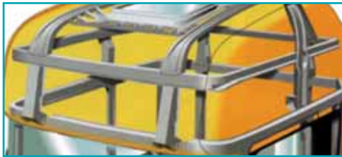
Structure of a truck cabin
