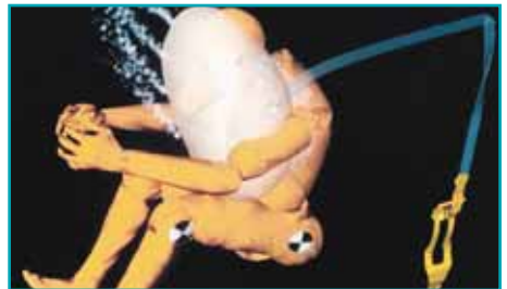
front airbag deployed
