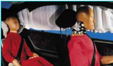
inflatable air curtain airbag
