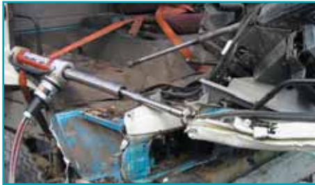
fully extended telescopic ram
