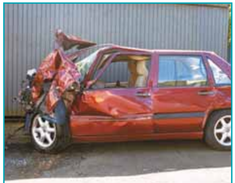
deformation due to crumple zones
