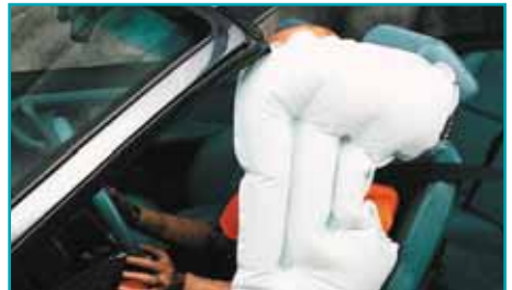
side impact chair mounted airbag
