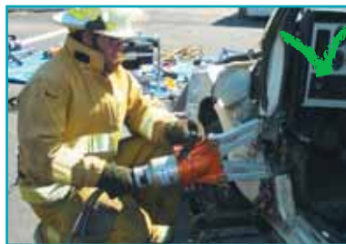
correct spreader positioning
