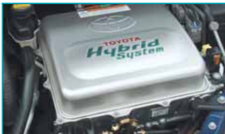
electronic drive system of Toyota “Prius”
