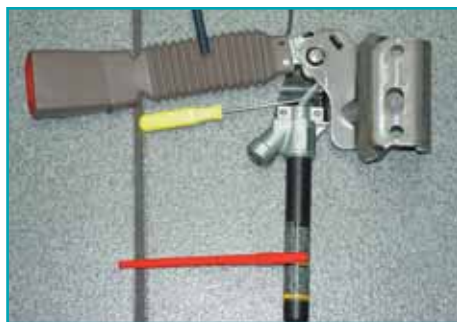
exposed seatbelt pretensioner
