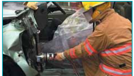
dash lift using ram
