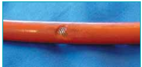
do not use damaged hose
