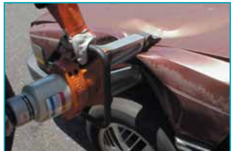
squeezing / crushing a fender
