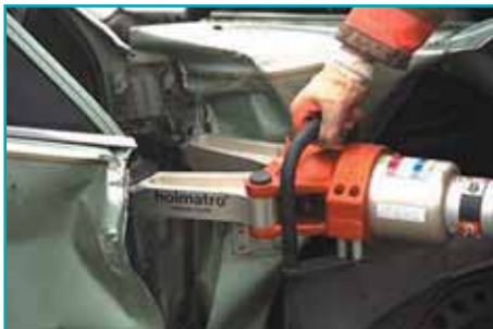
spreading a door from the vehicle
