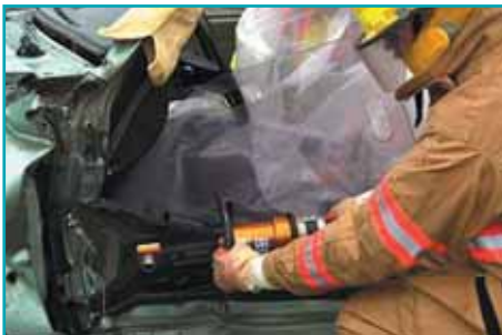
dash lift using combi-tool
