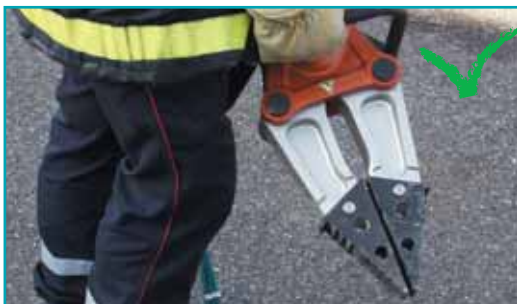
spreader carried correctly by handles
