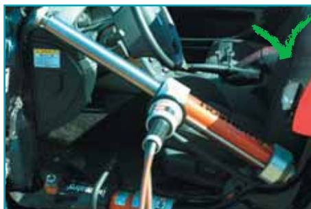
relief cut made before ramming starts
