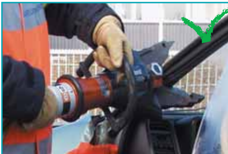
material far into blade recess
