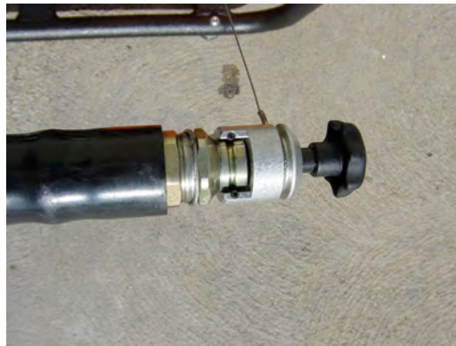
Male coupler w/ dust cap Pressure Relief Device in use
