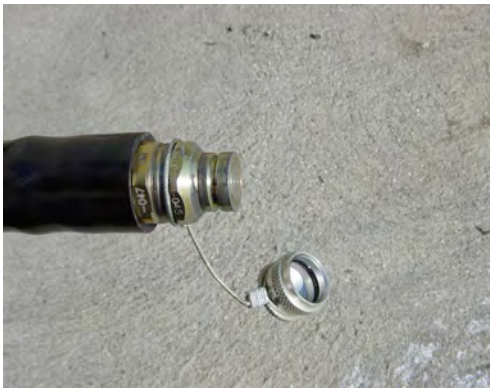
Male coupler w/ dust cap Pressure Relief Device in use
